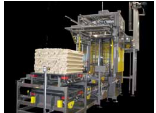
Bag depalletizer less partial pallet removal area and empty pallet stacker or magazine. This machine depicts a smaller footprint.
